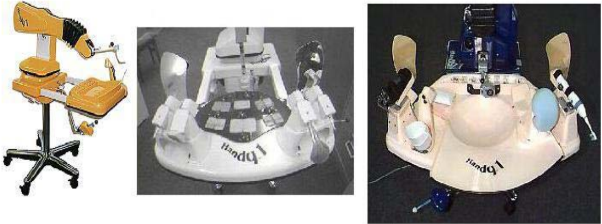
Figure 2.8 HANDY - for eating food, applying make-up and, brushing and shaving
