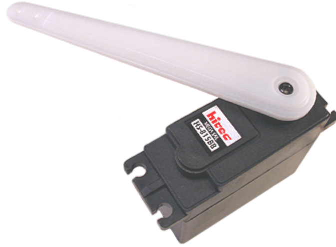
Figure 3.14 Servo for link 1
