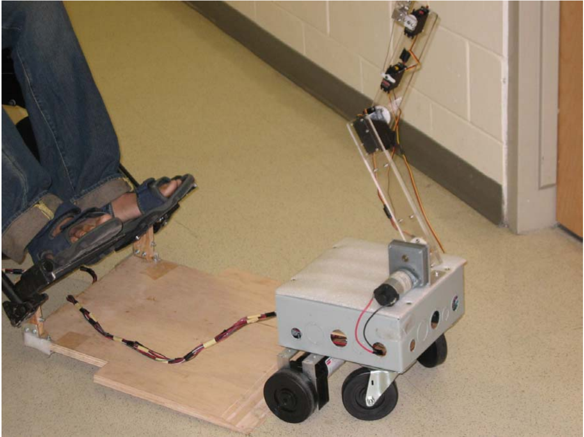
Figure 5.8 Robot climbing back after user has passed through
