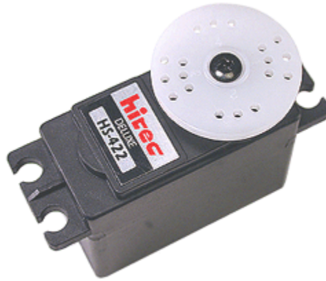
Figure 3.13 Servo for gripper and wrist
